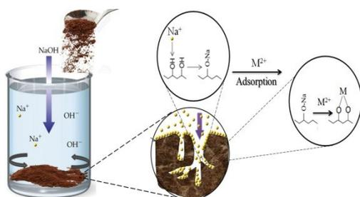
(decrease of hemicellulose content from 19.23% in KK to 3,52% in KKM; FT-IR spectrum shows loss of  $1730\text{ cm}^{-1}$  peak in KKM, that shows  $\text{-C=O}$  group in hemicellulose). FT-IR and SEM analysis showed that with alkaline treatment wax and oils are removed from the surface of the
